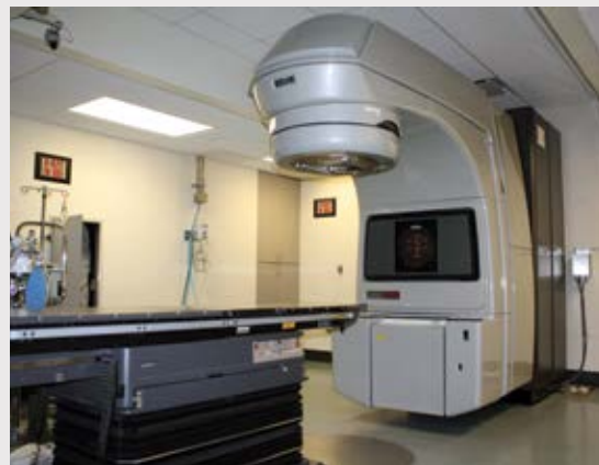
↳ The Varian 2100 C/D linear accelerator is able to rotate. A rotating field facilitates precision during treatment.
